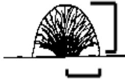
$$\text{Frontal Silhouette Area} = (3.14 \times \text{Maximum Height} \times \frac{1}{2} \text{Maximum Width}) \div 2 \text{Eq. 16}$$
