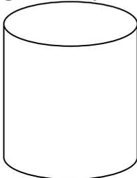
$$\text{Frontal Silhouette Area} = \text{Maximum Height} \times \text{Maximum Width} \quad \text{Eq. 14}$$
