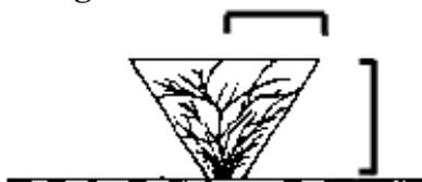
$$\text{Frontal Silhouette Area} = \text{Maximum Height} \times \frac{1}{2} \text{ Maximum Width} \quad \text{Eq. 15}$$
